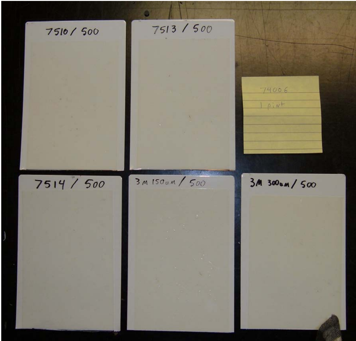
Figure 2 500 hr UV sample after 1 pint of stone impact
