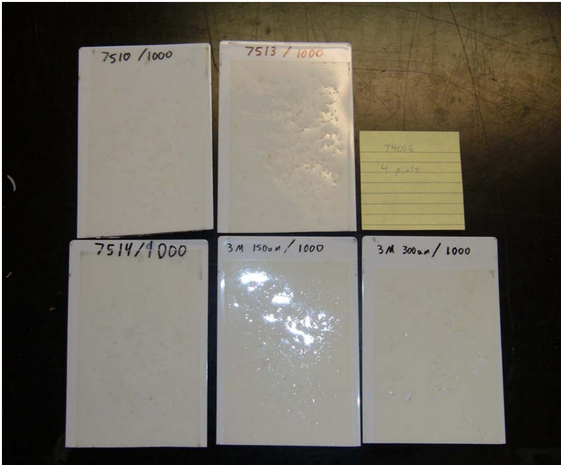
Figure 13 1000 hr UV sample after 4 pints of stone impact
