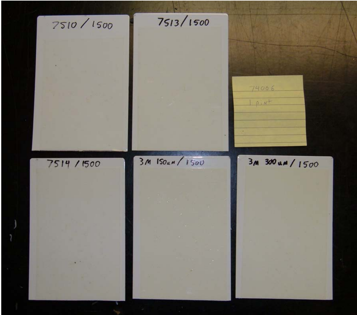
Figure 4 1500 hr UV sample after 1 pint of stone impact
