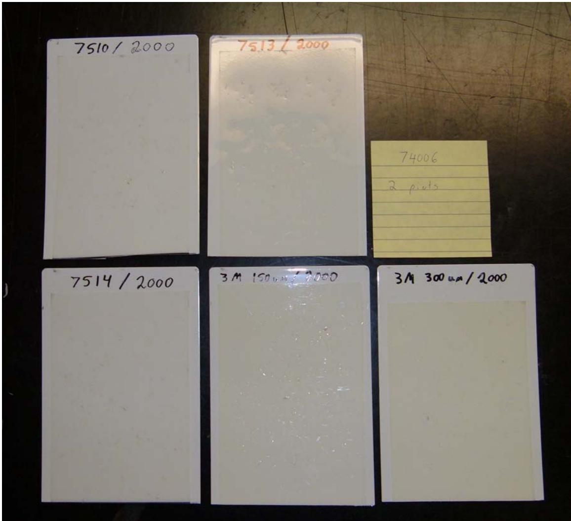
Figure 10 2000 hr UV sample after 2 pints of stone impact
