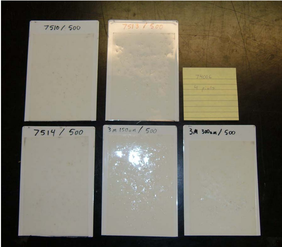
Figure 12 500 hr UV sample after 4 pints of stone impact
